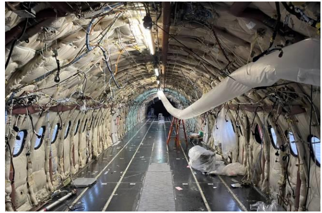
< Aircraft after passenger seats have been removed >
