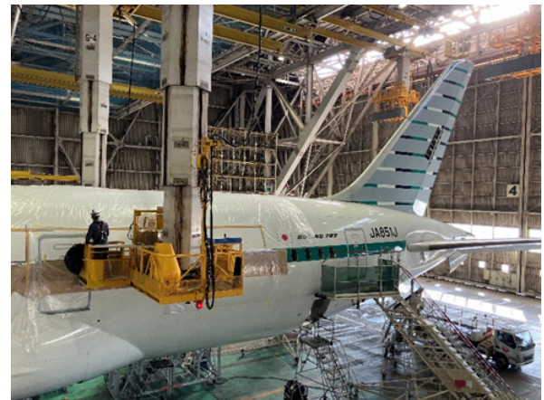
Riblet Application Work Scene at JAL Hangar, Narita International Airport
