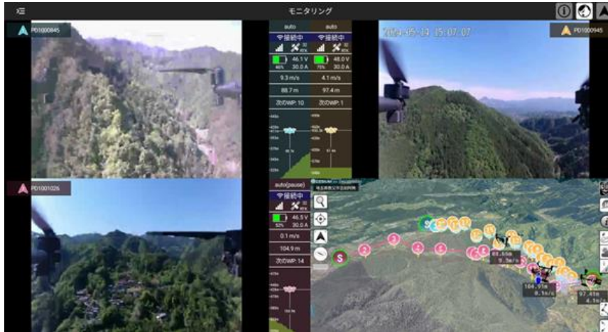
Operational management system screen: Develop an intuitive UI design for displaying information of multiple aircraft, with a layout that minimizes the need for shifting viewpoints.
