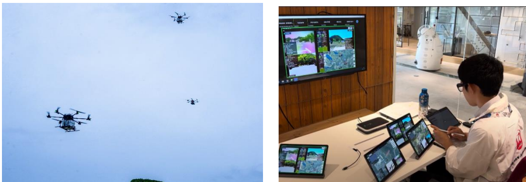
Scenes of Simultaneous Operation of Three Drones with a Single Remote Pilot
