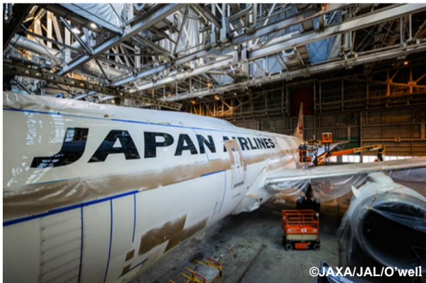
Riblet Application Work Scene
