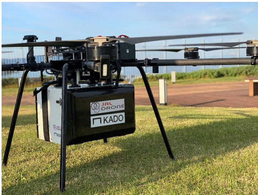
< Drone equipped with transport box provided by KADO >
